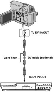
Video unit equipped with DV connector
